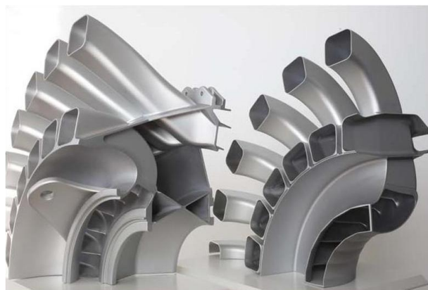
Figure 21: Models of Alternative Intercase Designs for an Intercooled Engine
