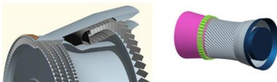
Figure 12: Sketch of variable core cycle study (left) and of innovative combustion with pulse detonation features (right)
