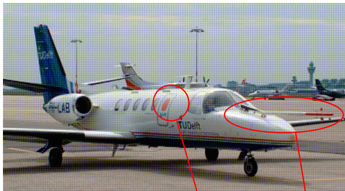
Figure 13: NLR's aircraft with laser window and nose boom
