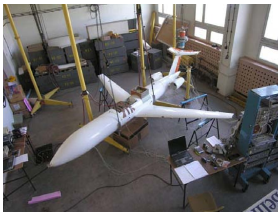
Figure 33: IEP 21 during vibration tests
