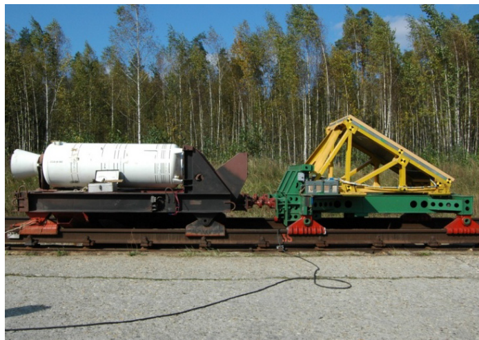
Figure 94: General view of the test bench with inclined screen for trolley speed 200-250 m/s
