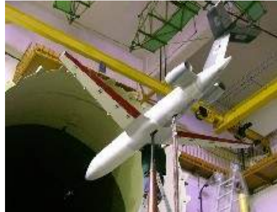
Figure 32: IEP21 Tested in the Wind Tunnel
