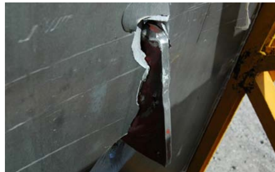
Figure 93: Step 1.3 Launch 1 impact (back side of target)
