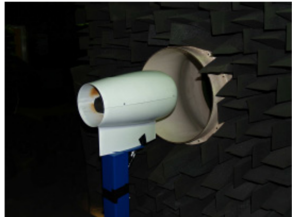
Figure 28: Assessment of nacelle's effects on noise emission
