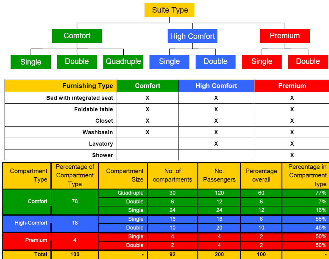
Figure 114: Definition of comfort level and number of cabin/sleeper compartments for the PDA
