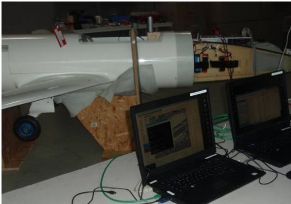
Figure 35: HIL tests of the IEP
