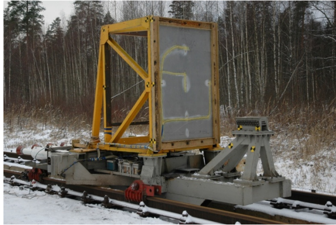
Figure 96: General view of the test bench with rotation device for trolley speed 100-150 m/s
