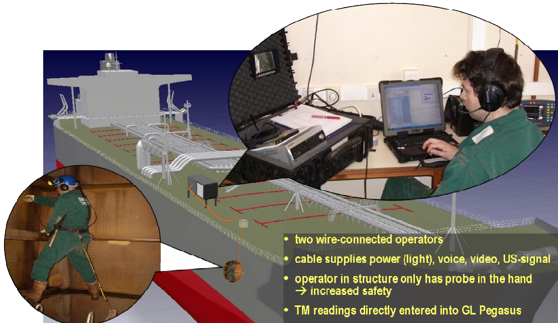
Fig.10: Data collection using a direct connection between UTM equipment and GL Pegasus
