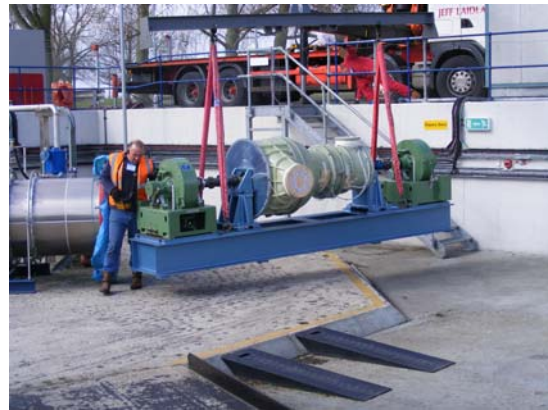
Turbine and Dynamometers on Bed Plate [D3.2.5]
