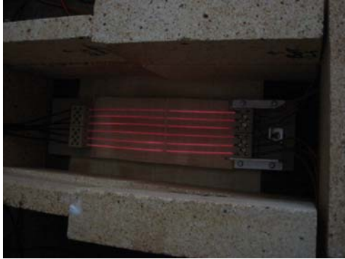
Oxidation testing of Inconel 718 tubes
