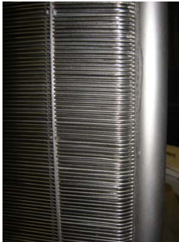
Close-up of pre-cooler matrix/header brazed joint
