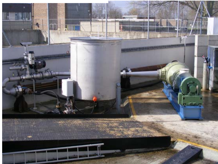
Complete turbine test rig. In the foreground is the 5 ton hot water tank and the water feed pump. In the background is the argon supply system and to the right the turbine and dynamometers.
