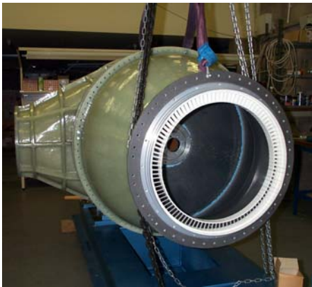
Turbine inlet casing
