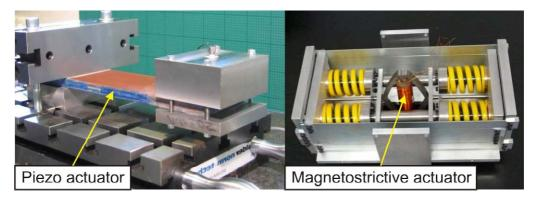
Experimental testing of piezoelectric force generator for vibration reduction on helicopters including its power supply. The desired forces could be generated at the specified frequencies;
