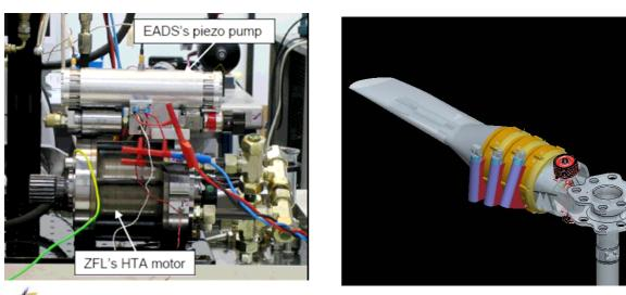
Tests of both smart pumps produced in laboratory environment with artificially simulated loads;
