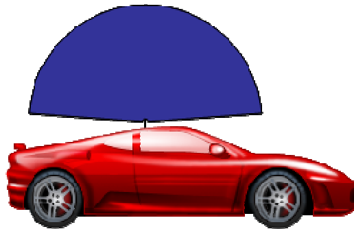
Figure 4-10: Roof-top antenna with almost hemispherical coverage
