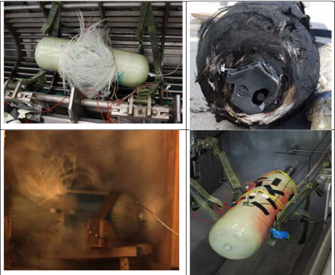
Figure B1.1: Extensive testing was performed by BAM and WRUT of the new vessels. (Shown, clockwise from top left: Burst tests, fire engulfment, bullet penetration, and AE-testing)
