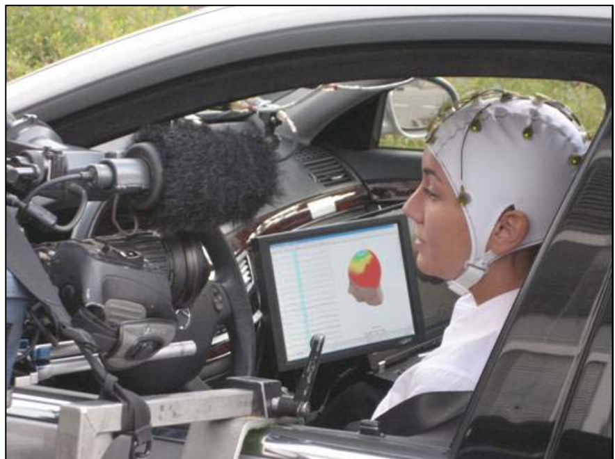
Daimler "Brain Cap" experimental setup with door-mount camera
