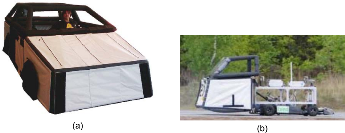
Figure 11 The ASSESSOR, standalone (a) and rear part mounted on propulsion system (b)
