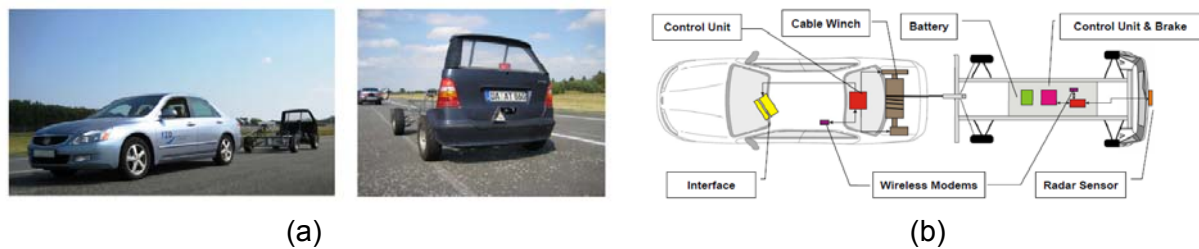
Figure 15 The EVITA target (a) and its design (b)
