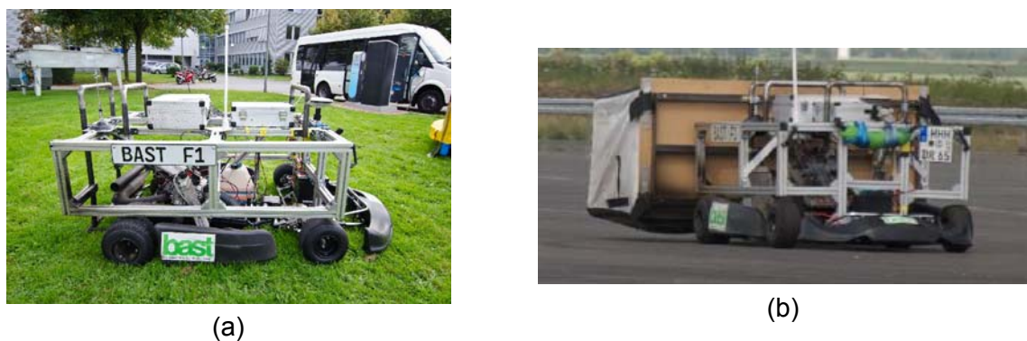
Figure 12 The Marvin propulsion system, without (a) and with (b) rear-end target
