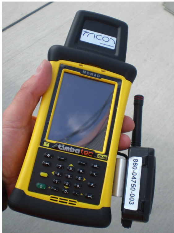
Fig. 30: CHINOS handheld with integrated container RFID tag and eSeal reader
