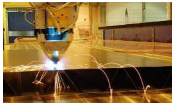
Figure 4.1-3 - laser welding head (from www.schulergroup.com/en/30products/80laser_technology/20PEDILAS/index.php )
