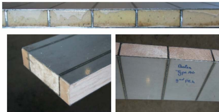
Figure 4.2-4 – all-metal sandwich panels filled with adhesively-bonded solid block materials.
