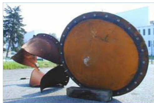
Figure 8.1-8 – hybrid metal sandwich: SPS, with possibly enhanced robustness for a military environment, developed by Intelligent Engineering.
