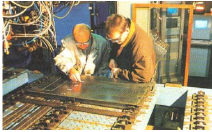
Figure 6.1.1.1-1 - direct visual inspection of laser welded I-Core panels.
