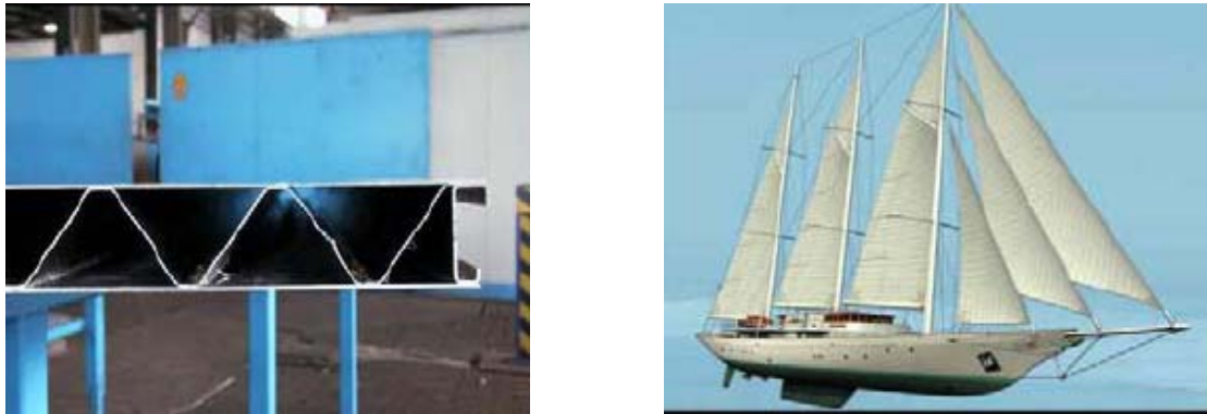
Figure 2.2-4 - application of CORALDEC™ panels in the mega yacht Athena built in the Netherlands.
