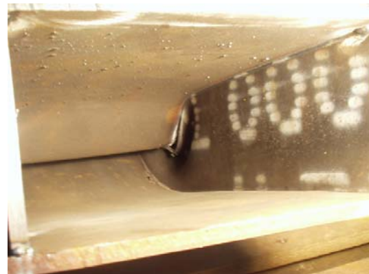
Figure 6.1.1.1-5 – an endoscope image from inside an I-Core sandwich panel.
