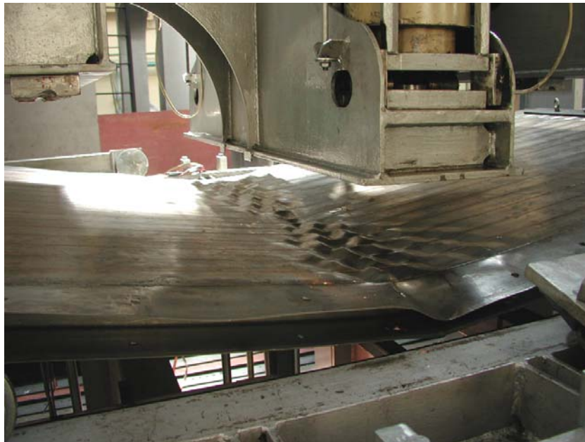
Figure 3.1.2.3b-4 – I-Core panel following testing showing mode of failure.
