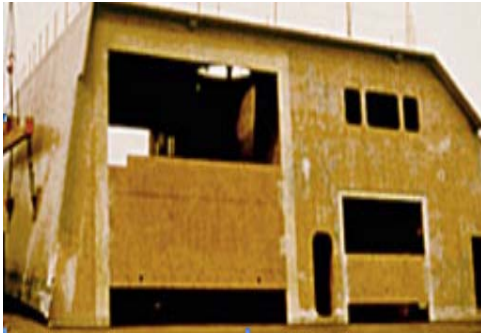
Figure 8.1-5 - composite sandwich: fibreglass (GRP) facings and balsa wood core, as applied for the helicopter hangar of the French naval vessel La Fayette.
