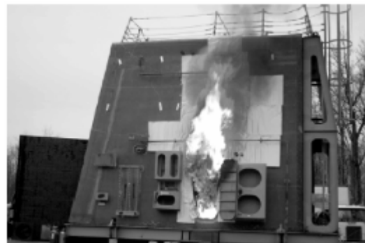
Figure 2.4-5 - fire testing of a prototype composite sandwich helicopter hangar under the US Navy's Libra programme. Extensive trials demonstrated that fire was not a major problem provided that composite structures were well-protected.
