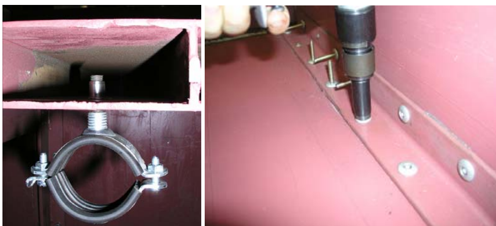
Figure 5.2-7 - bolted connection (left) and riveting (right) to the faceplate of an all-metal sandwich (Henkel et al. 2005).
