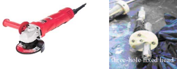
Figure 6.2.2-2 - typical grinder (left) and water jet lance (right).
