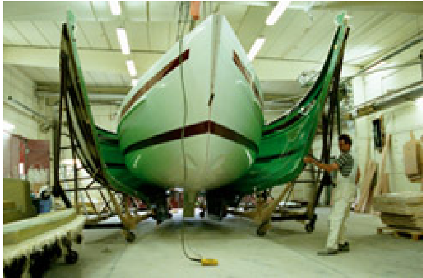
Figure 5.1.3-2 - boat hull being removed from a mould.
