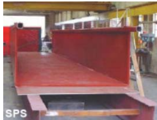
Figure 2.3-2 - mid-ship section of a barge (SPS – steel facings and polyurethane elastomer core).
