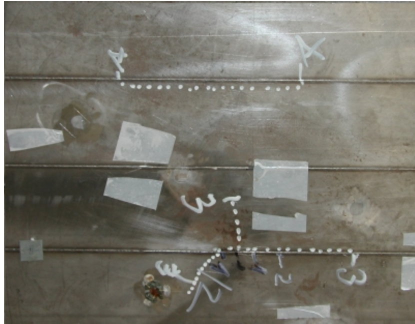
Figure 3.3.2-2 – specimen A: fatigue crack propagation paths.
