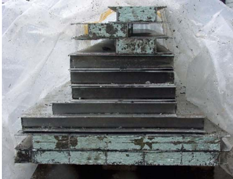
Figure 4.2-2 – all-metal sandwich panels filled with light concrete.
