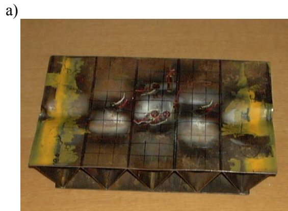
Figure 3.1.2.1b-1: a) buckling and b) denting of the top faceplate.
