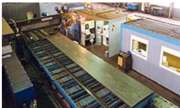
Figure 4.1-2 - gantry and sliding table (from www.i-core.com )
