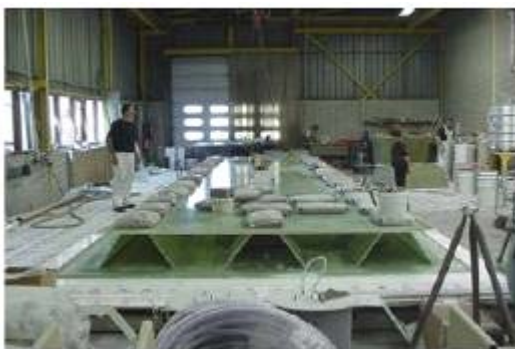
Figure 2.4-4 - prototype grain bulkhead produced by the Technical University of Delft. A weight saving of 50-70% compared to an equivalent steel structure was realised.
