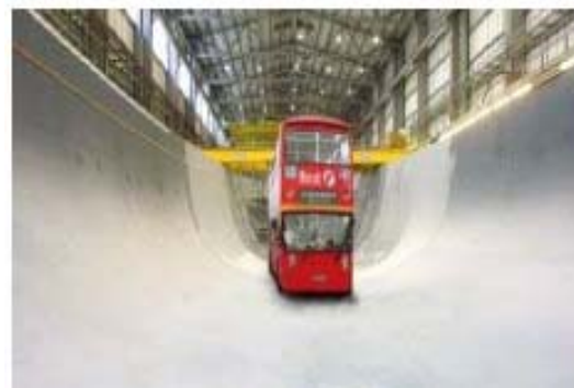
Figure 2.4-3 - hull of the Mirabella V yacht, the largest marine composite structure produced to date at 75 m long. The sandwich construction used for the hull and deck consists of glass reinforced vinylester facings and a polymer foam core. Carbon and aramid fibre reinforcements were also selectively employed.
