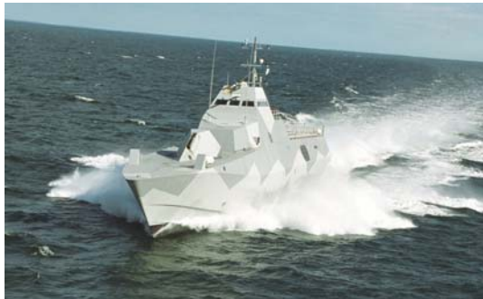
Figure 8.1-6 - composite sandwich: carbon fibre reinforced polymer (CFRP) facings and polymer foam core, as applied to the Swedish naval vessel Visby.
