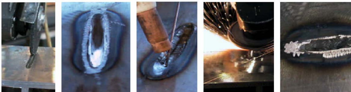
Figure 6.2.1-1 - repair of an all-metal sandwich. From left to right: (i) grinding on top of the laser weld, (ii) panel after grinding and chiseling, (iii) TIG repair welding, (iv) grinding after repair welding with a Polyfan-Disc, (v) repaired panel after welding and grinding (from Reinert 2002).
