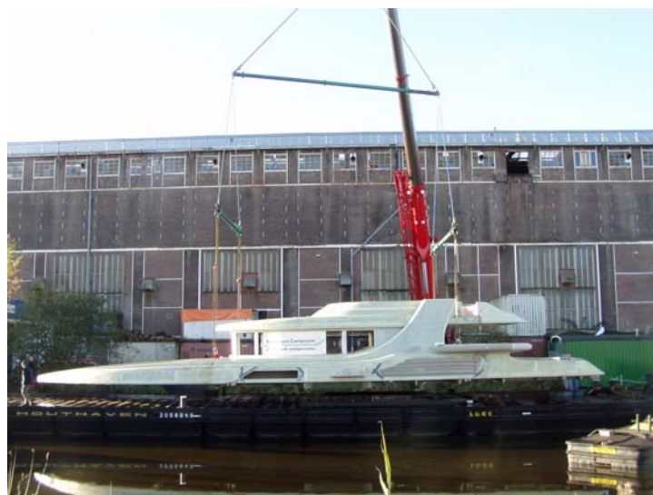
Figure 5.2-1 - sandwich superstructure for a luxury yacht produced from carbon/glass fibre reinforced epoxy facings and a polymer foam core (Rhebergen Composiet Constructies).
