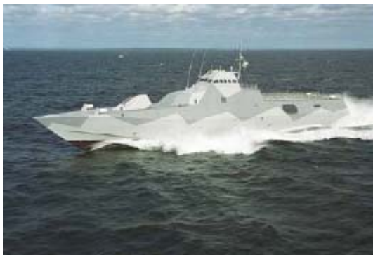
Figure 2.4-2 - hull of the Visby class corvette – carbon fibre reinforced polymer facings and PVC foam core.
