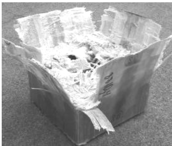
Figure 3.2.3-2 - a hollow rectangular composite sandwich tube following progressive crushing (from Pitarresi et al. 2006).
