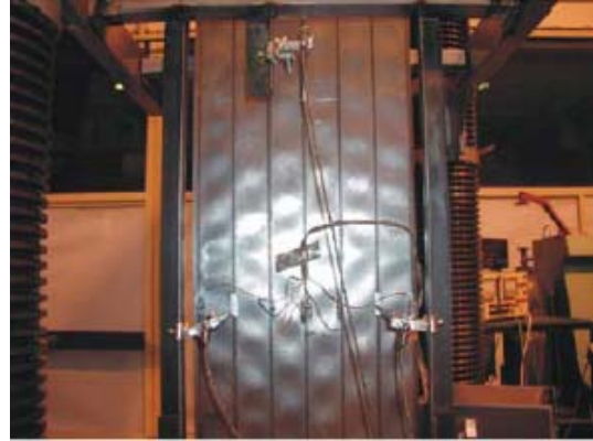
Figure 3.1.3.3-6 – local buckling deformation over an entire faceplate.
