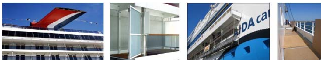
Figure 8.3-4 - prefabricated balconies by Joptek (pictures on left) and Meyer Werft (pictures on right).
