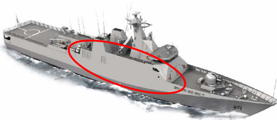
Figure 8.1-2 - selected superstructure module, part of the SIGMA offshore patrol vessel developed by Schelde Naval Shipbuilding.
