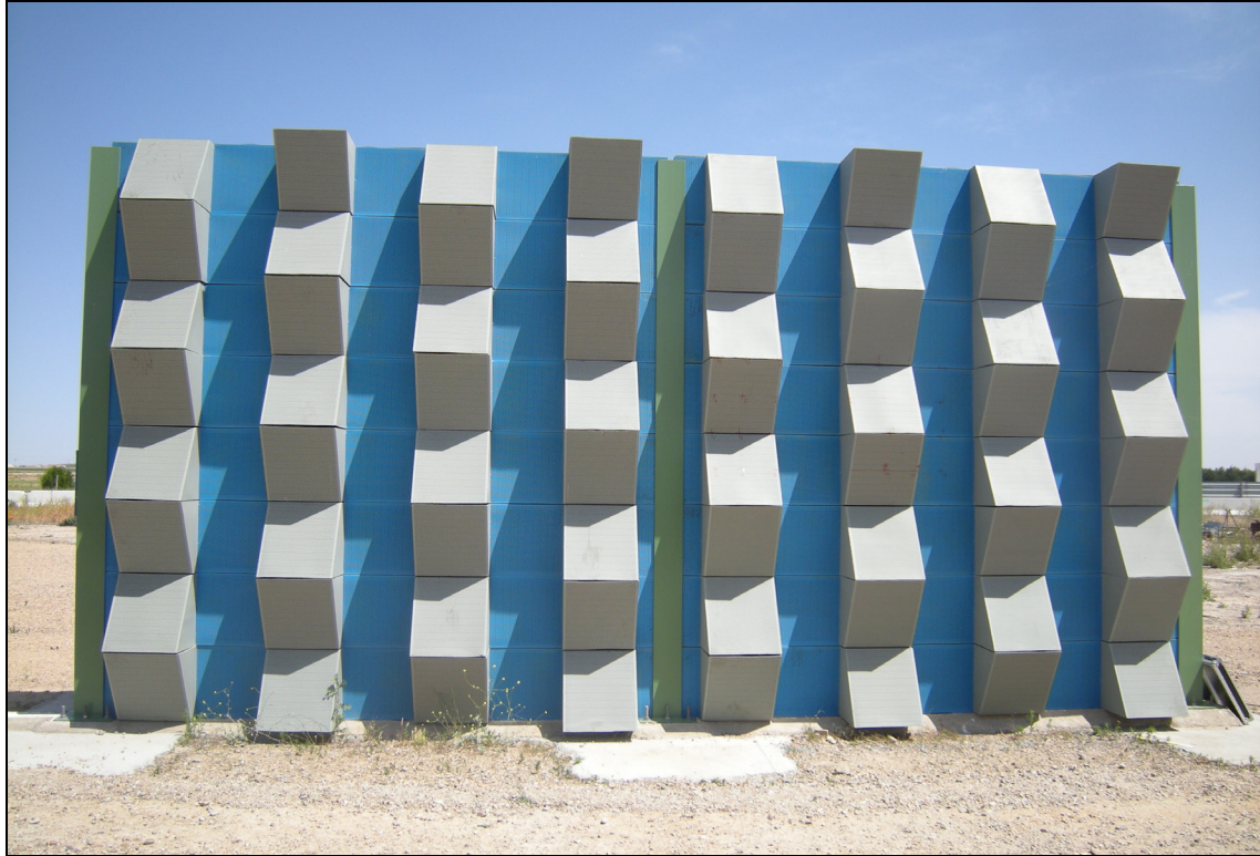
Fig. 5 – Sample 1 (strongly non flat, sound absorbing) on the Valladolid test site.
