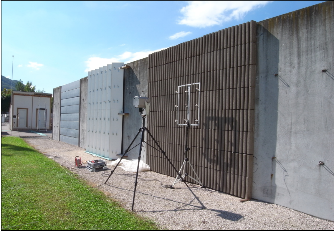
Fig. 7 – Sample 3 (gently non flat, sound absorbing) on the Grenoble test site.
