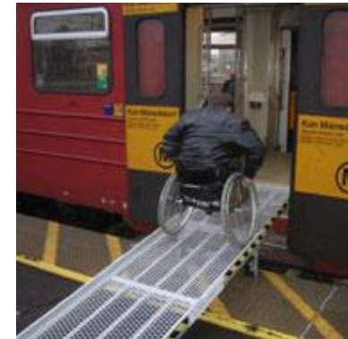
Manual ramp, Norway
