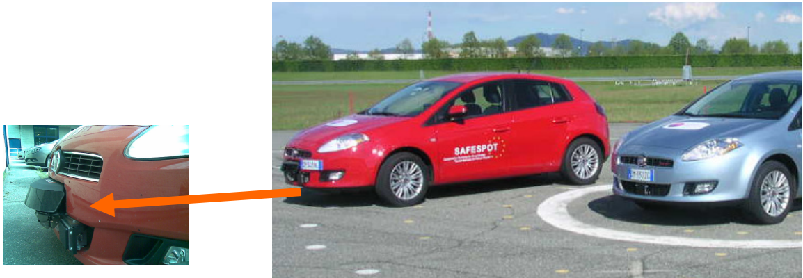
Figure 31: The SAFEPROBE (details of Laser Scanner and Radar) and SCOVA vehicles
