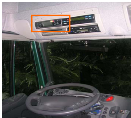
Figure 57: Tractor OBU integrated in truck cabin.
