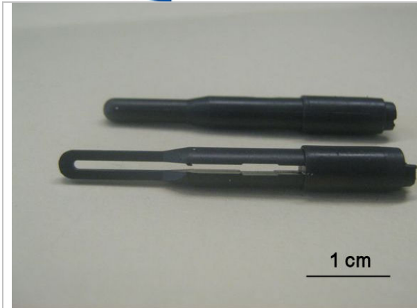
Fig. 1 Glow plugs in the green state
