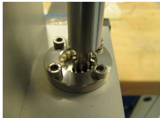
Figure 8 Results of torque measuring tests with ten gear wheels and measuring device
