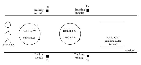
Figure 34 – Sensor fusion of multiple imaging subsystems to determine successively the risk level of a person
