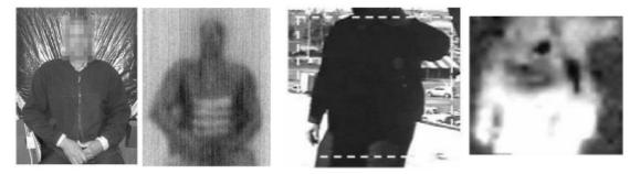
Figure 29 – Passive mm-wave image taken (left) indoor, and (right) outdoor
