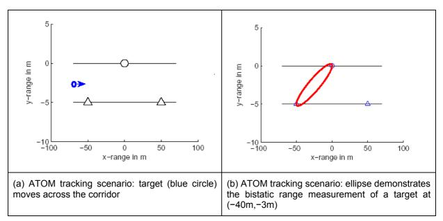
Figure 39 – Tracking scenario: Corridor with two sources (triangles) and a single passive receiver (circle); target moving across the corridor is shown by blue circle.
