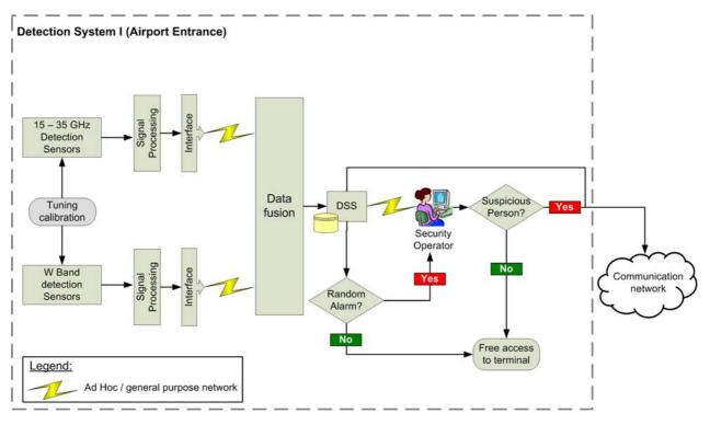
Figure 23 – ATOM Architecture: Detection system I (Airport entrance)
