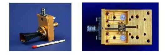
Figure 9 – The radar modules of the 3-D millimeter wave luggage scanner
