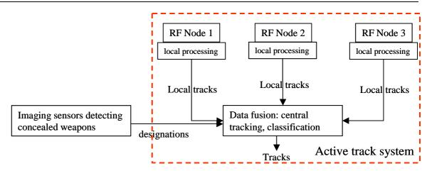
Figure 44 – Schematic overview active tracking system
