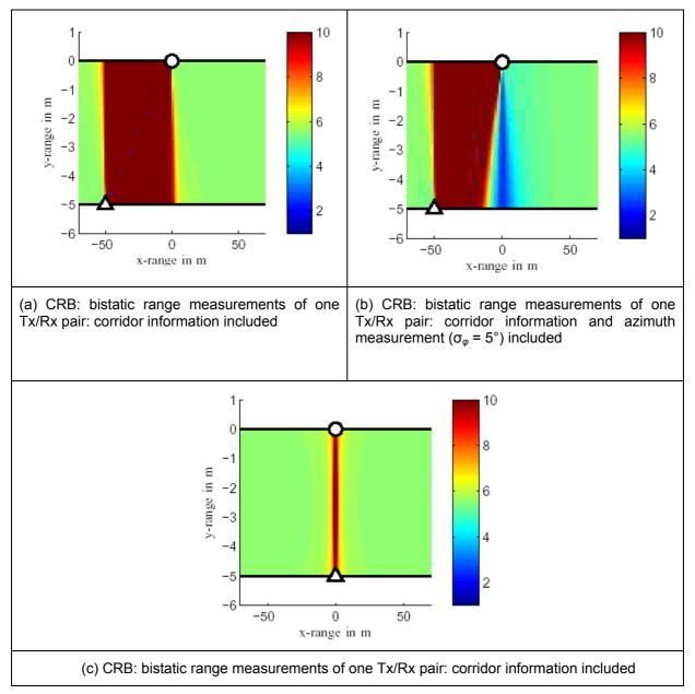
Figure 41 – CRB of position estimate (one Tx/Rx pair)
