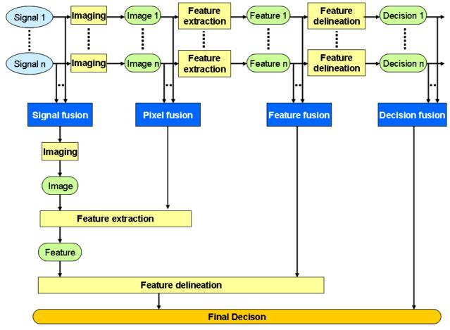
Figure 51 – Processing levels of image fusion
