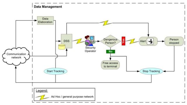
Figure 26 – ATOM Architecture: data management block
