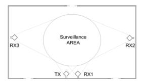
Figure 37 – Typical displacement for a network of receivers in a Passive Radar System
