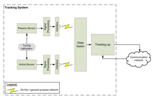
Figure 25 – ATOM Architecture: tracking system block
