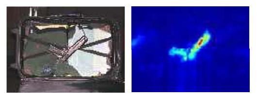
Figure 10 – The picture of a two dimensional scan about a suitcase containing a firearm
