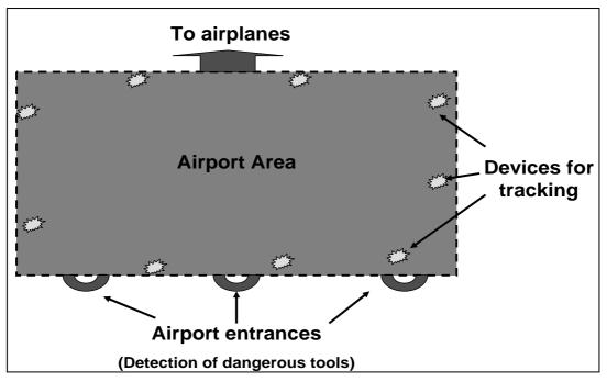
Figure 21 – Distribution of the detection and tracking sensors of ATOM system in the airport area
