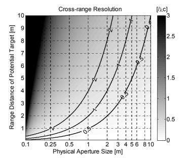
Figure 27 – Cross-range resolution of two-way array under variant physical aperture size and range of target
