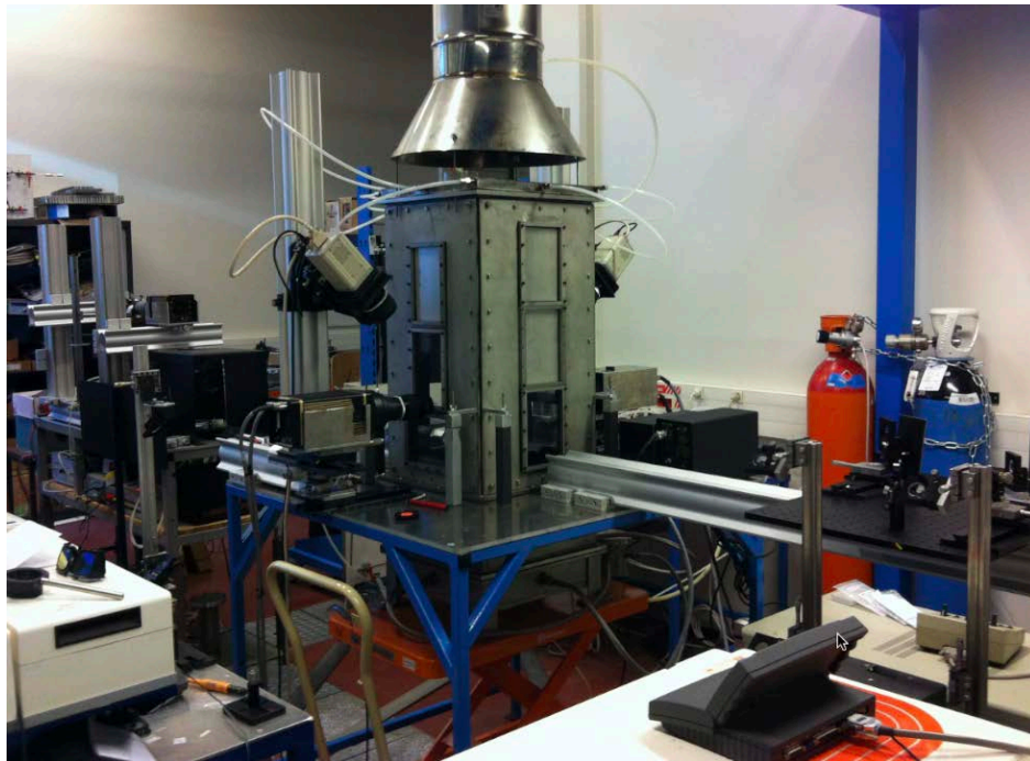
Figure 4.1 – Configuration set-up of SPIV and double-pulsed OH fluorescence technique on the burner at CORIA laboratory (CNRS PC2A/LML/CORIA)
