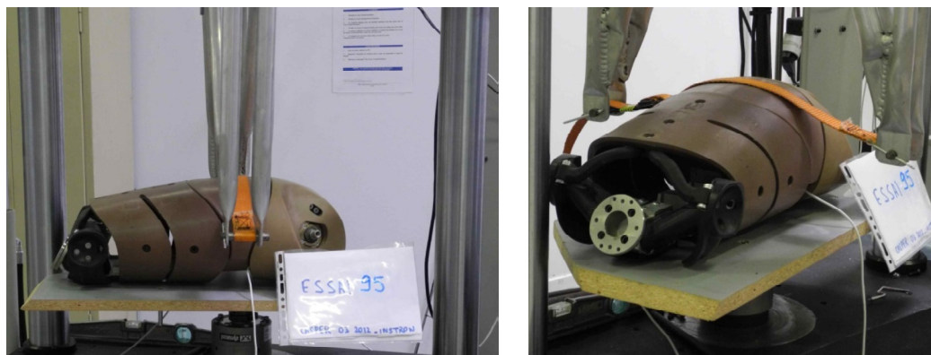
Figure 4-35: Belt compression tests: illustration of the test setup for the Q10 dummy
