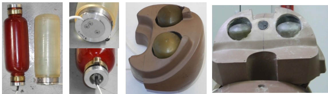
Figure 4-34: Left: APTS V1 (small diameter cap, darker colour) and V2 (large diameter cap, light colour). The APTS are approximately 50mm in diameter. Right: APTS V2 inserted in a Q3 and in a Q10 abdomen. The V2 was used for the current study
