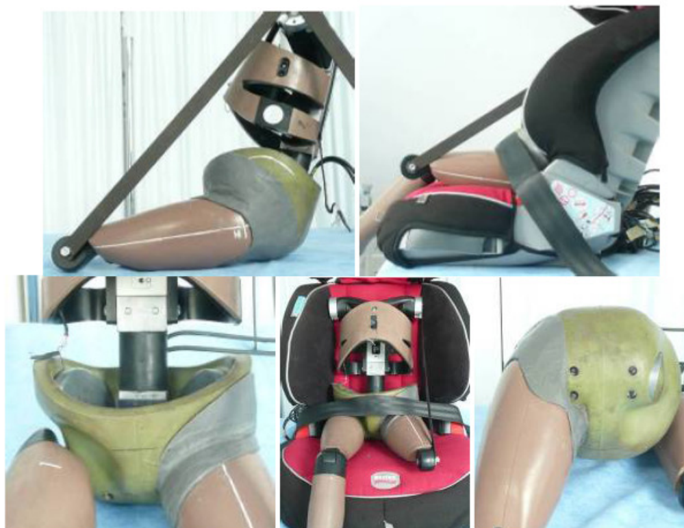
Figure 4-23: Insert model (in grey plastiline) at the pelvic-thigh junction - the insert was modelled in a reference position that was maintained using a rigid bar In this design, the insert goes around the complete thigh while leaving the access to the hip screws (bottom right)
