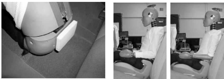
Figure 4-8: Position of the Hill 6YO dummy in a booster seat (Reed et al. , 2006) Left: proposition of padding to help positioning the dummy. Centre: posture without padding. Right: posture with padding
