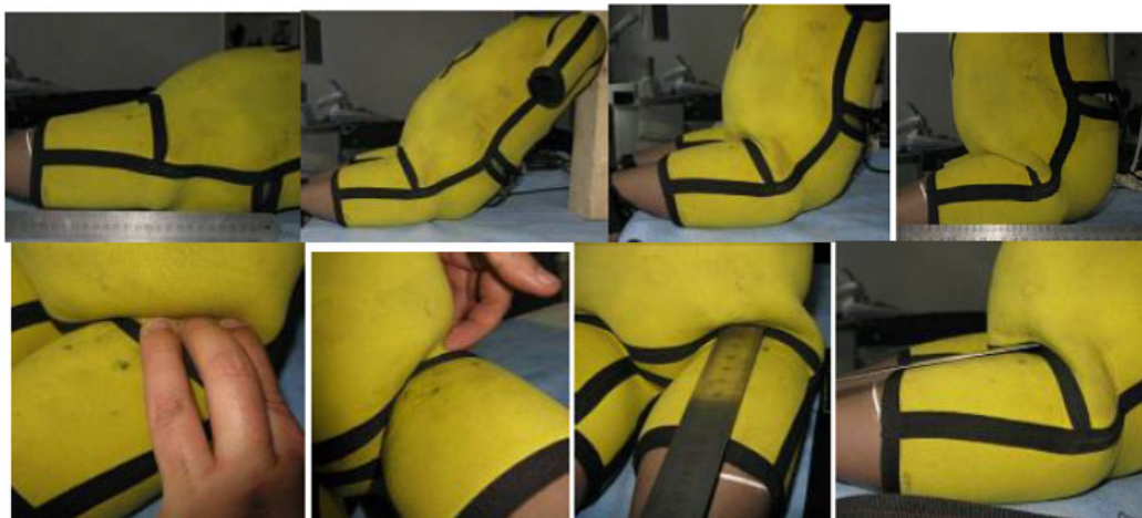
Figure 4-17: Q3 dummy with suit: effect of hip angle on the fold at the groin
