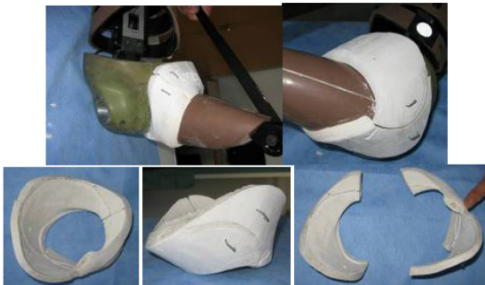
Figure 4-24: Illustrations of the plaster mould build around the plastiline insert and the dummy
