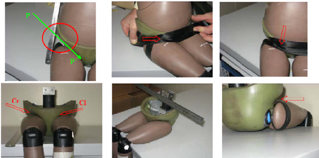
Figure 4-16: Illustration of the gap at the pelvis-lumbar junction (groin): dummy without the suit.
