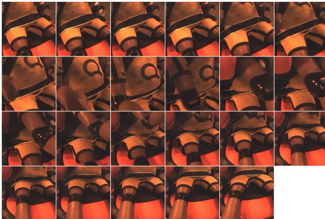
Figure 4-31: Lap belt kinematics in standard position with the silicon insert (test 11) the overall kinematics is similar to the response without auxiliary equipment. Based on the rebound images, the belt does not appear to penetrate the gap and does not really fold. It remains stable on the pelvis thigh gap during the complete kinematics
