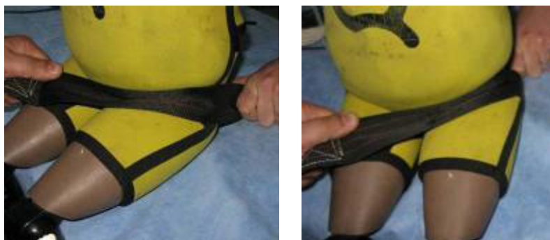
Figure 4-18: Gap and belt penetration with suit. Under manual tension, the belt seems to be able to penetrate the gap (front and side)
