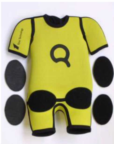
Figure 4-27: Illustration of the Q3 dummy jacket modified by FTSS
