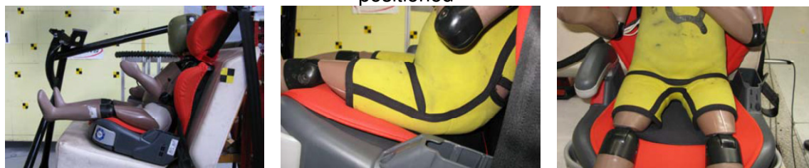
d) Left: silicon inserts (without the suit); Center and right: close-ups of the area without silicon inserts installed. Notice how the inserts fill the gap and removes the folds
