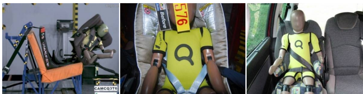
Figure 2-20: Misuse of CRS fixation (left), misuse of restraining child in CRS (centre), misuse of seatbelt restraining the child (right)
