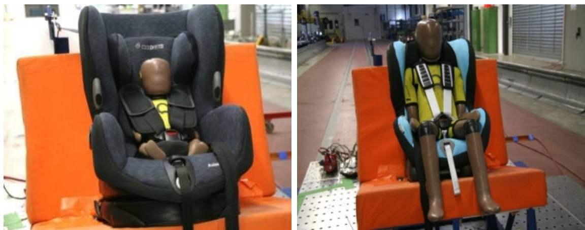
Figure 2-21: Inappropriate use Q0 (left) and Q6 (right) in a G1 harness CRS
