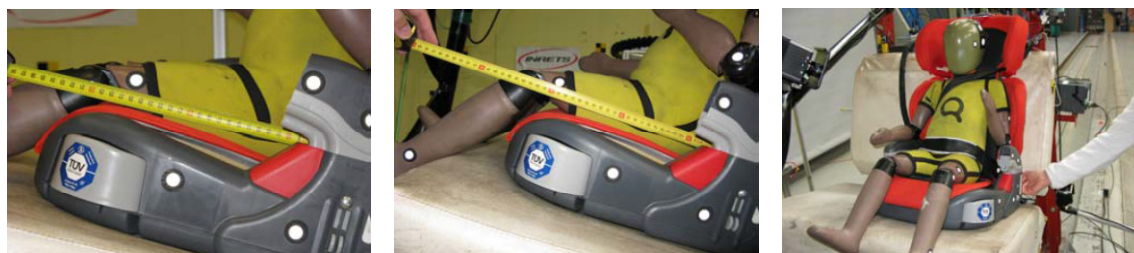
e) Left: Standard position (11) with the back against the seat; Centre: Relaxed position (12) until the knee clears the front of the seat; Right: misuse (the belt does not pass around the armrests)
