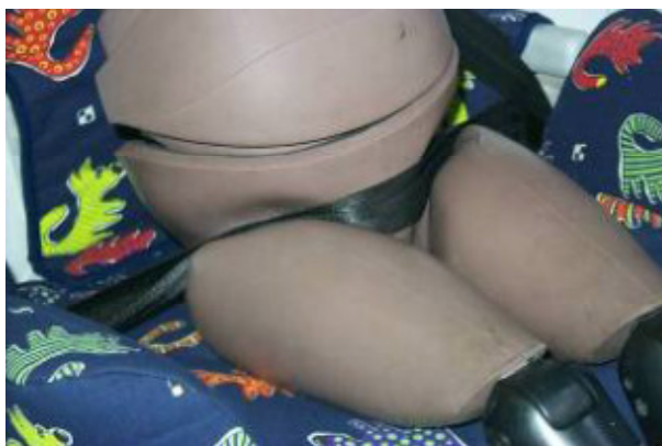
Figure 4-9: Illustration of potential problem with the groin (Johannsen Goubel, 2004) (The neoprene skin is removed for a better visualization of the phenomenon)
