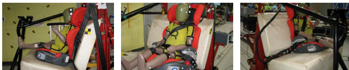
a) Overview of the setup (no auxiliary equipment) prior to the testing - Notice the fold in the dummy suit
