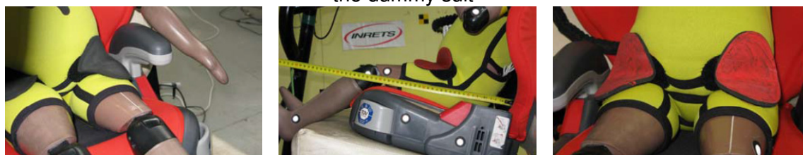
b) From left to right: Softest (not tested), medium (6) and thick (8) patches positioned. The patches tested were painted in red and the belt was highlighted with white
