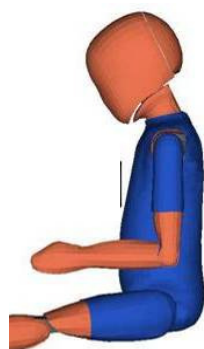
Thorax shape from lateral view, slope of the thorax facilitates in addition to the shoulder design upwards movement of the shoulder belt
