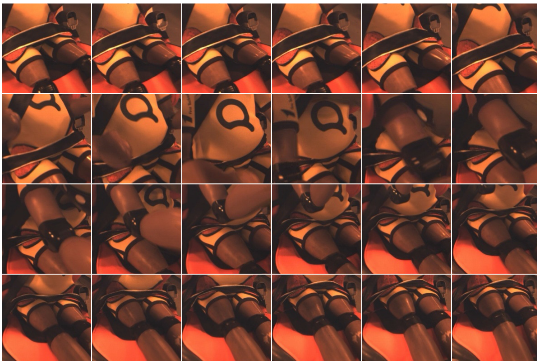
Figure 4-30: Lap belt kinematics in standard position with the thick patch (test 8) The overall kinematics is similar to the response without auxiliary equipment. Based on the rebound images, the belt does not appear to penetrate the gap (bottom rows). The belt gets folded longitudinally during the dummy flexion and remains folded after the rebound.
