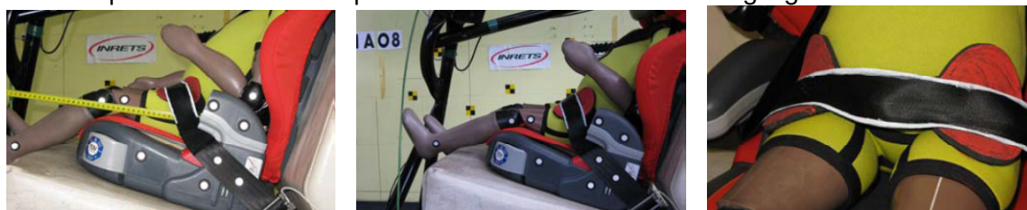
c) From left to right: Medium (6), thick (8) and thick close-up (9) patches with the belt positioned
