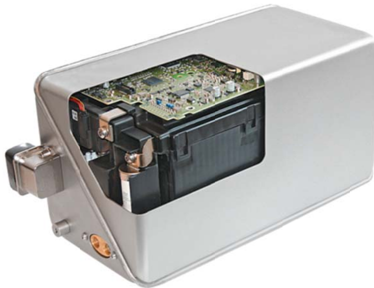
Figure 21. - Lithium Ion Energy Storage System with overall BMS outside the battery-cell pack
