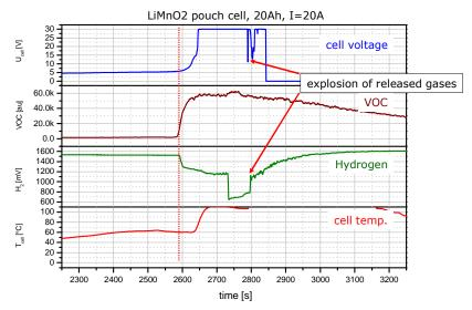
Overcharging experiment with cell venting followed by explosion of released gases.
