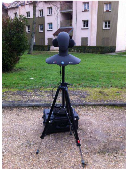
Figure 3 : Head Acoustic Dummy with windscreen
