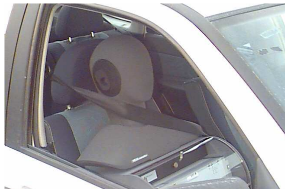
Figure 9. Position of the binaural acoustic head in the reference vehicle for the measurement of interior noise (passenger position).
