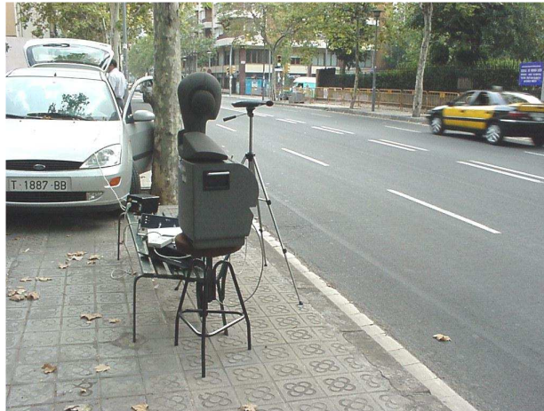
Figure 7. Preparation of the set-up for the measurements with the artificial head ( Paseo Bonanova - Barcelona )
