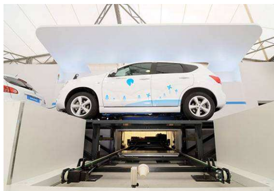
Figure 16 – A vehicle on a Better Place battery switch station [2]
