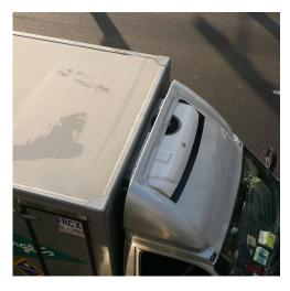
Figure 4: Well-adjusted deflectors reduce fuel consumption
