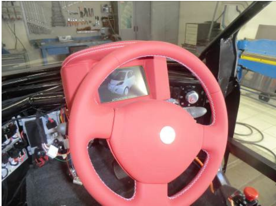
Fig. 20: Front view of display, steering wheel and engine selector
