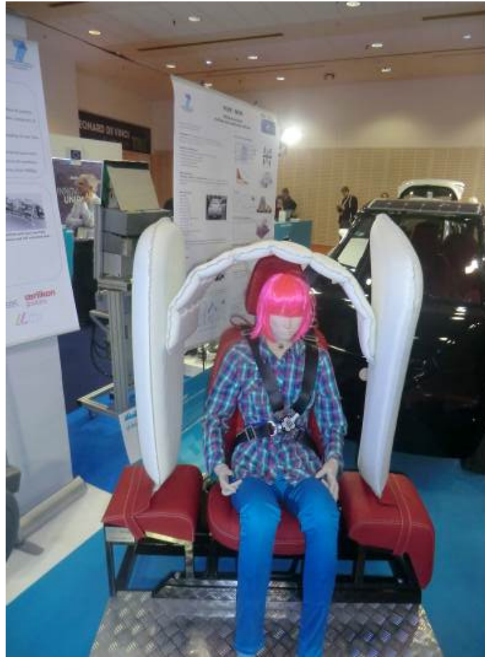
Fig. 24: Demo of front seat airbag system protection
