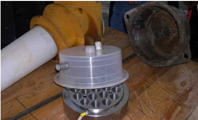
Figure 7: Transparent cap of the anchor head used in the prefabricated elements of the segments of Piacenza Viaduct (Foto V. Nicollier [19])
