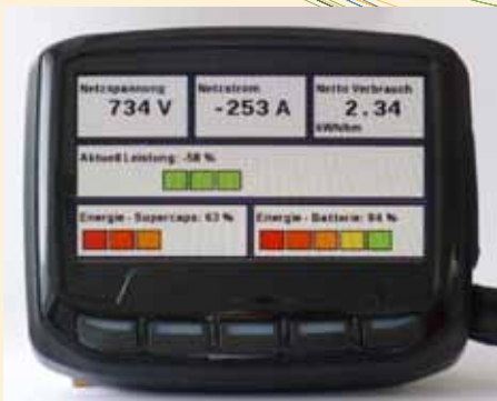
Illustrations of IT-eco-driving assistance displays tested in Eberswalde and Parma
