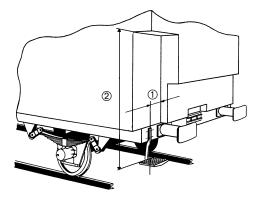
On wagons fitted with shock-absorbers, the areas marked with black and yellow stripes must also remain clear.
