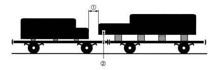
A clearance of 10 cm from the floor should be respected when the load protrudes beyond the end axles or bogie centres of the carrier wagon by no more than 6.5 m.
