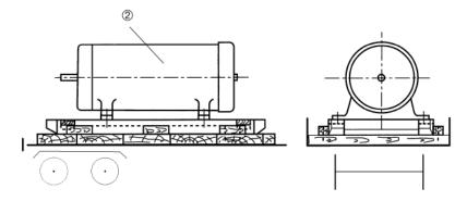
To prevent lateral movement of the load and the resulting encroachment of the loading gauge, and/or to ensure the 1.25:1 ratio between the loads per wheel is not exceeded, the goods should be secured laterally. The provisions of sections 5.4.1 and 5.4.3 should also be observed.
