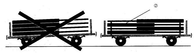
Stacks formed of cylindrical units may be loaded in flat tiers or in dovetailed formation.
