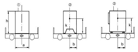
These values shall also apply if goods on cradles, sleds, etc. are bound together to form a single load unit.
