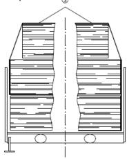
For low-density goods such as sawn timber, bindings with a breaking strength of 700 daN are permitted on an exceptional basis.
