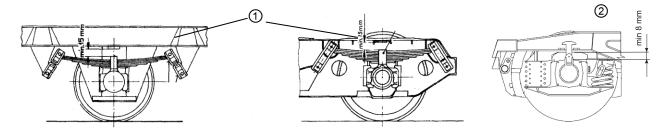
2 • the distance between the axle box and the bogie frame is < 8 mm.
