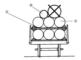
For stacks loaded on flat wagons and liable to sway laterally (e.g. metal trellis-work), the minimum horizontal clearances between the loading gauge and the load should be increased, as shown in tables 2.
