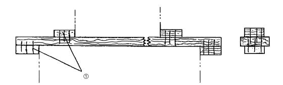
When attaching scotches used for cylindrical goods (for example steel pipes), the scotches must be the same width as the timbers to provide sufficient width for nailing and to prevent the scotches from splitting. Scotches should be nailed from both inside and outside; to this end, the securing devices should be prepared prior to loading.
