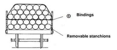
When fastening a load directly or indirectly, the fastenings may only be attached to the stanchions if the stanchions are secured against lifting.
