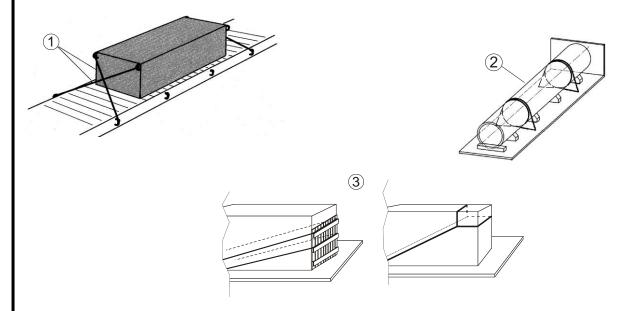
Direct fastenings placed lengthways in the wagon may be considered correctly dimensioned if the breaking strength<sup>2)</sup> (straight pull) of the bindings in each direction is at least
