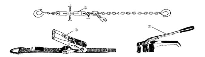
The locks and buckles of the securing straps must be adapted to the type of strap being used in terms of its functional properties and strength.
