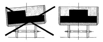
The permitted limit values for the differences between wheel loads are complied with when the centre of gravity of the load is transversally distant from the centre of gravity by no more than
