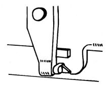
Where cylindrical goods are loaded in stacks or in dovetailed formation and lean against the removable stanchions so that they protrude by more than half their height, facing stanchion pairs should be joined together with bindings.
