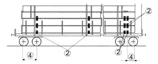
Timbers that are placed across the wagon and are liable to slide, for example during the loading of rails or steel profiles, must be secured against movement. To prevent them from hitting the stanchions in the event of longitudinal movement of the goods, timbers should be placed approximately half-way between adjacent sets of stanchions.
