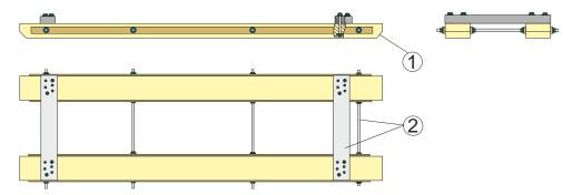
The goods should be fixed to the sliding timbers or trestles such that they are unable to move on it and are not in contact with the wagon floor.
