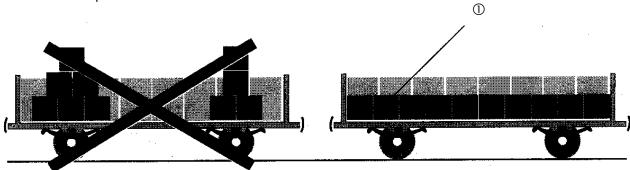
Superimposed units must form stable stacks that must be prevented from falling apart, for example by:
