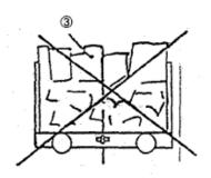
3 Light and heavy goods of this kind must not be made to protrude in order to increase the effective height of the walls.
