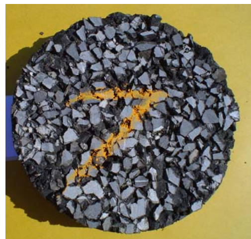
Figure 7. 2: Cross section of the old porous asphalt core from canton Aargau AG2
