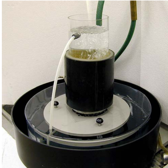
Permeameter; set up for horizontal measurements)
