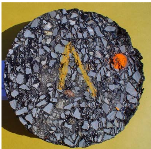
Figure 7. 1: Cross section of the new porous asphalt core from canton Aargau AG3
