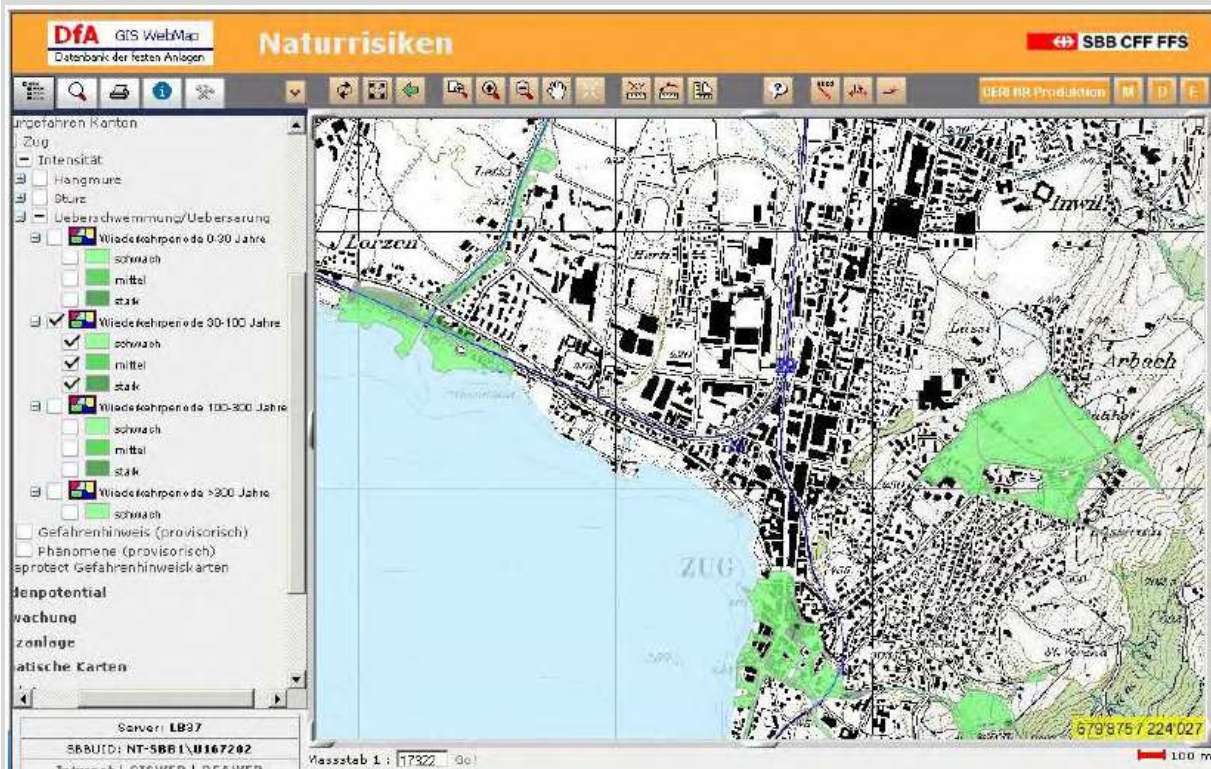
Figure 9: Example for a hazard map: Flooding hazard in Canton Zug in Switzerland for a return period of 30-100 years.
