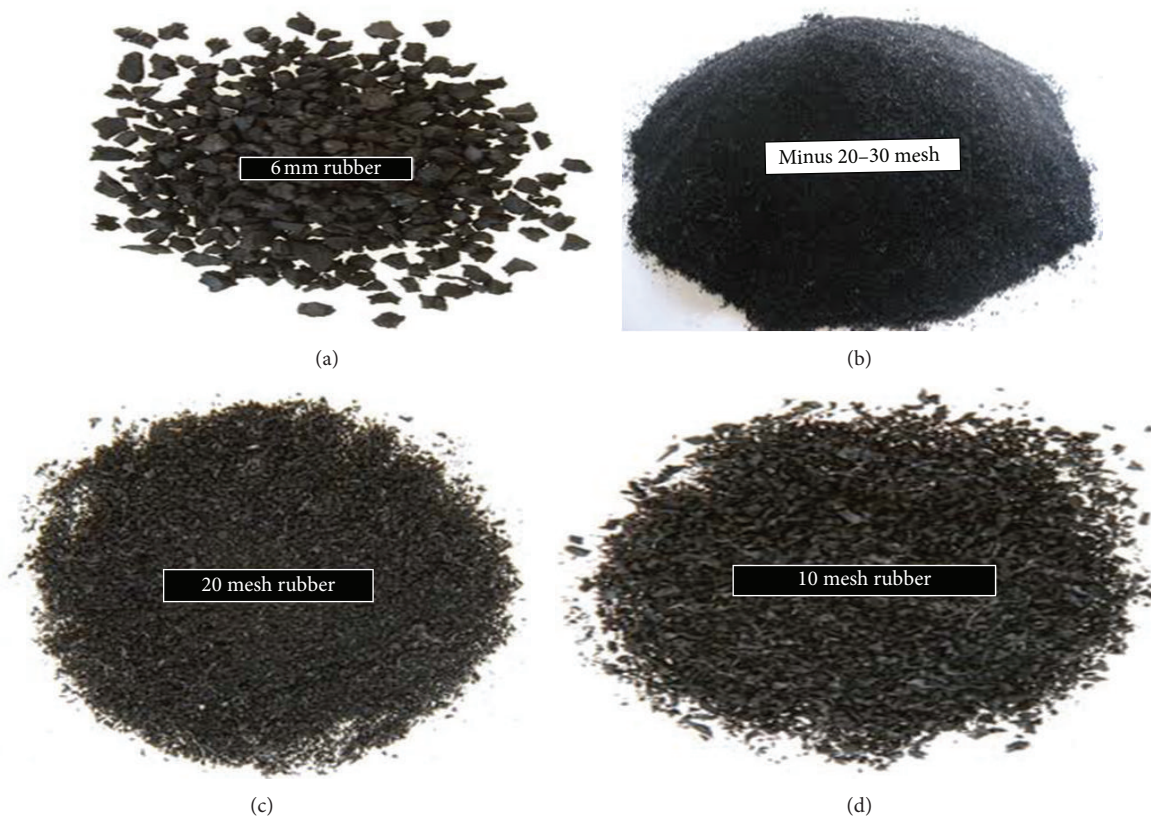
FIGURE 9: Different type of crumb rubber based on particle size.
