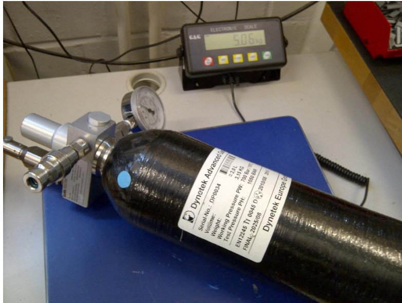
Figure 8: GHR valve/regulator and Dynetek cylinder (700 bar)
