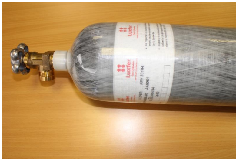
Figure 9: VTI valve/regulator and Luxfer cylinder (300 bar)
