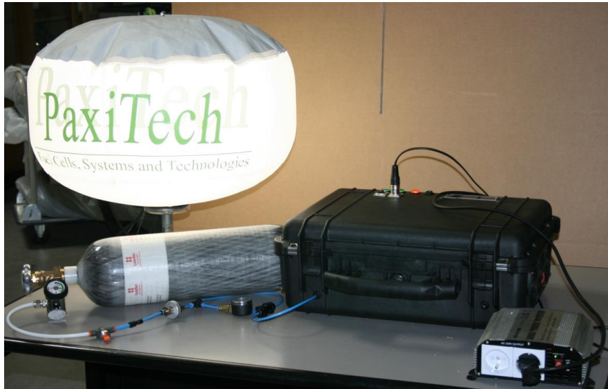
Figure 16: View of the fuel cell system powering a lighting balloon
