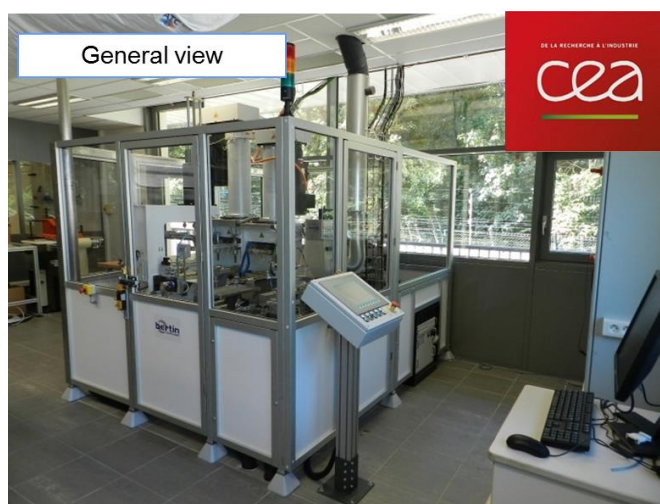
Figure 4: CEA's automatic machine for MEAs manufacturing.
