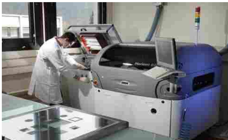
Figure 3: screen printing used for gas diffusion electrode manufacturing.
