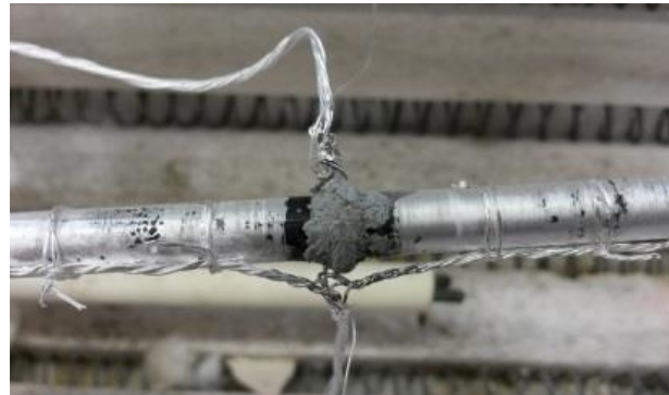
Ny/MT sealant silver degradation, but still acceptable performance
