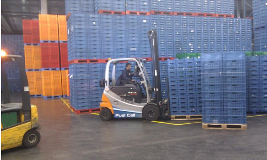
Figure 3: STILL RX60-25 FC at work, Colruyt Distributiecentrum Dassenveld
