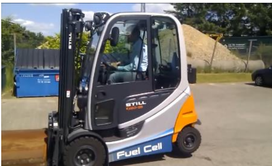
Figure 7: STILL RX60-25 FC excessive brake testing, H2 Logic
