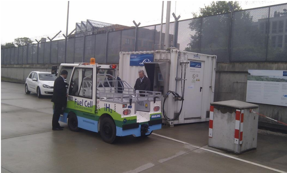
Figure 6: MULAG Comet 3FC on trial at Hamburg airport
