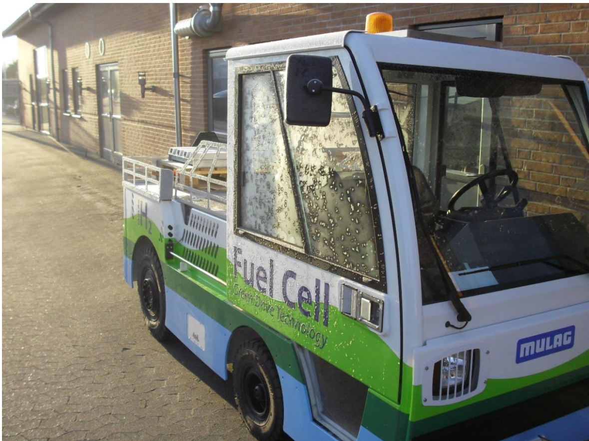
Figure 1: Climate tests of MULAG 3FC in winter @ -13°C
