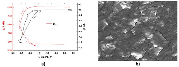
Figure 2. Voltammogram of La electrodeposition from an organic solvent. The red curve shows the resonance frequency change of the quartz resonator. One of the two Au electrodes (one on each side of the resonator) served as working electrode, onto which the La was deposited. The lowering of the resonance frequency clearly demonstrates successful deposition. b) Electron microscope image of a layer formed after transfer through air.
