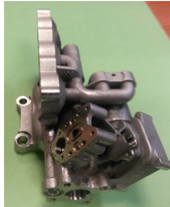
Housing after conventional finishing process
