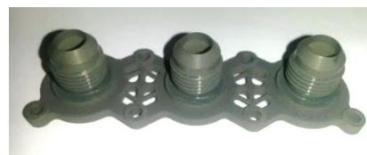
blank of connector holder – aluminum additive manufacturing
