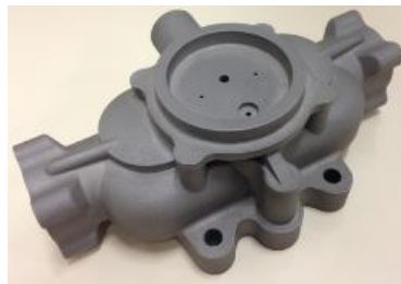
Additive manufacturing housing (works at technological brick level)
