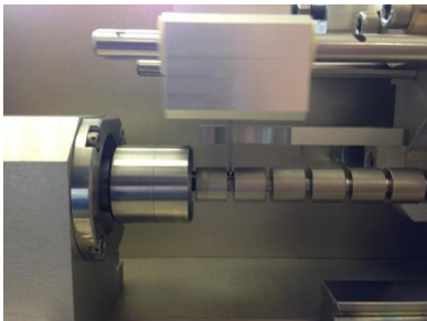
Tribologic test bench dedicated do reproduce contact ball / spool in accelerated conditions
