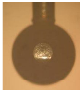
wear effect seen on ball on EHSV
