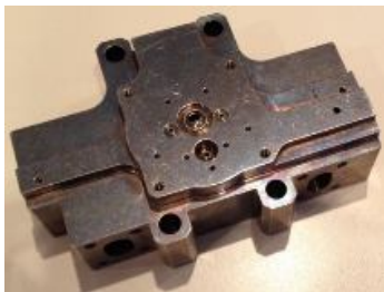
Conventional manufacturing housing (demonstrator engine SV)
