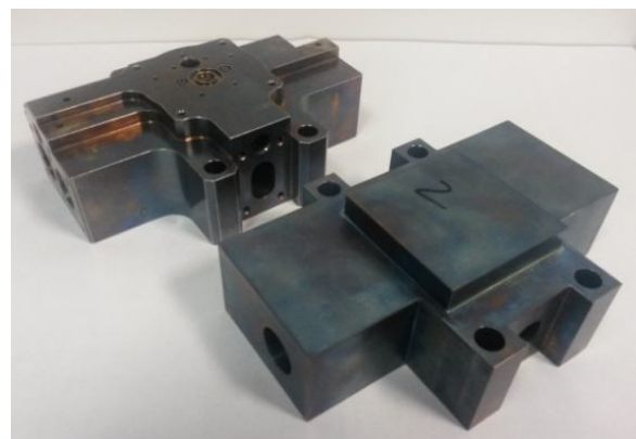
“Simplified housing” used for finishing machining tests
