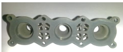
blank of connector holder – aluminum additive manufacturing
