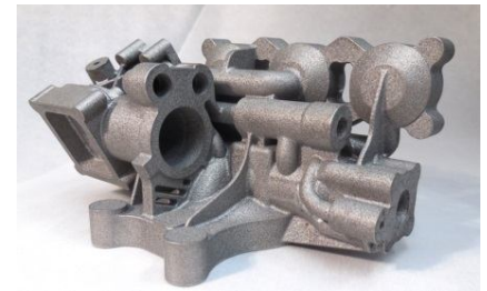
Additive manufacturing housing (target engine SV)
