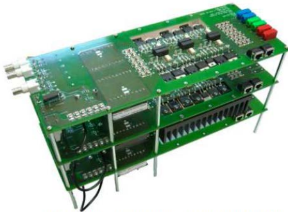
10kW TRU (INDRA and CEI-UPM): Three interleaved rectifiers.
