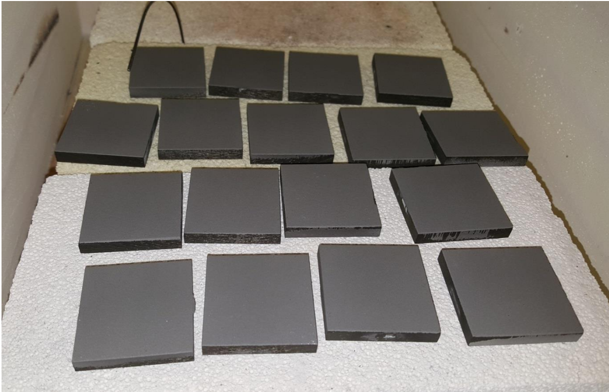
Figure 6: Coated composite panels inside oven during long exposure testing (200°C for 750hr)
