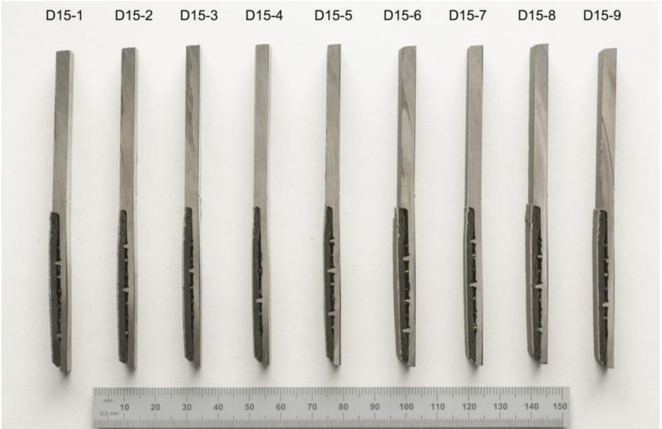
Figure 10: Representative visual examination of the SEDs after mechanically tested
