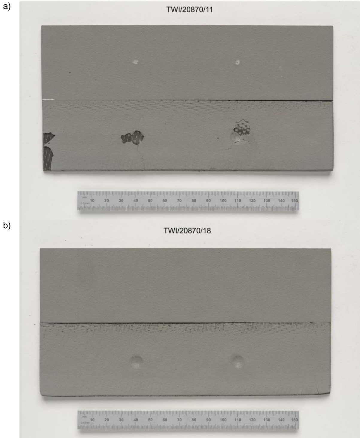
Figure 8: Coated SEDs after impact testing using a method based on ASTM D2794. a) SED TWI/20870/11 D2 after impact testing. One impact per area was applied to the coated Ti alloy, 2 impacts per area were applied to the CFRP. b) SED TWI/20870/18 D5 after impact testing of the CFRP. One impact per area was applied to the coated CFRP. All impacts had energy of 17.64J
