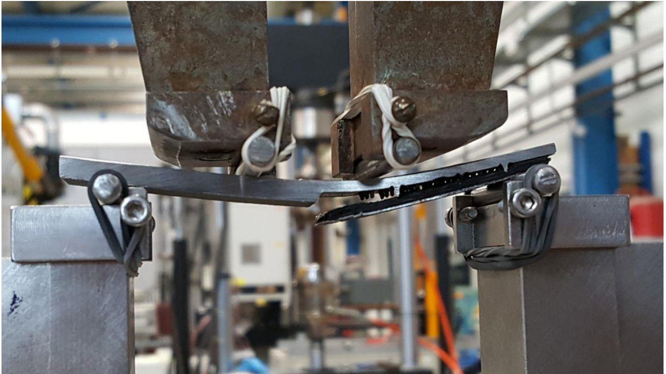
Figure 9: 4-point bending test of sub-element demonstrator
