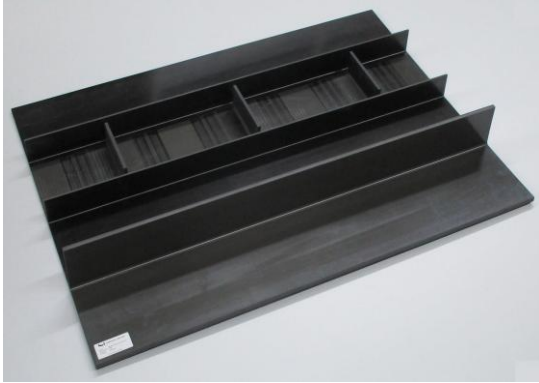
Figure 1: Finished stiffened panel
