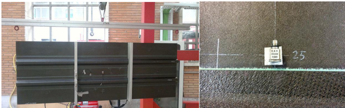
Figure 8. Left) Dynamic test set-up; right) detail of accelerometer bonded to the specimen
