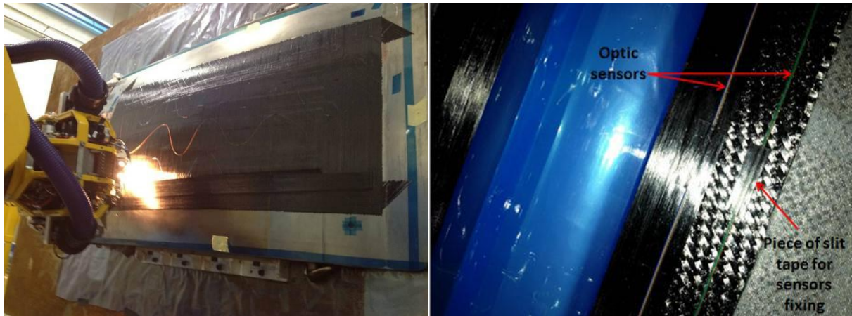
Figure 6. Left) automatic slit tape positioning over optic sensors integrated in the skin, right) positioning of optic sensors in the feet of stringers
