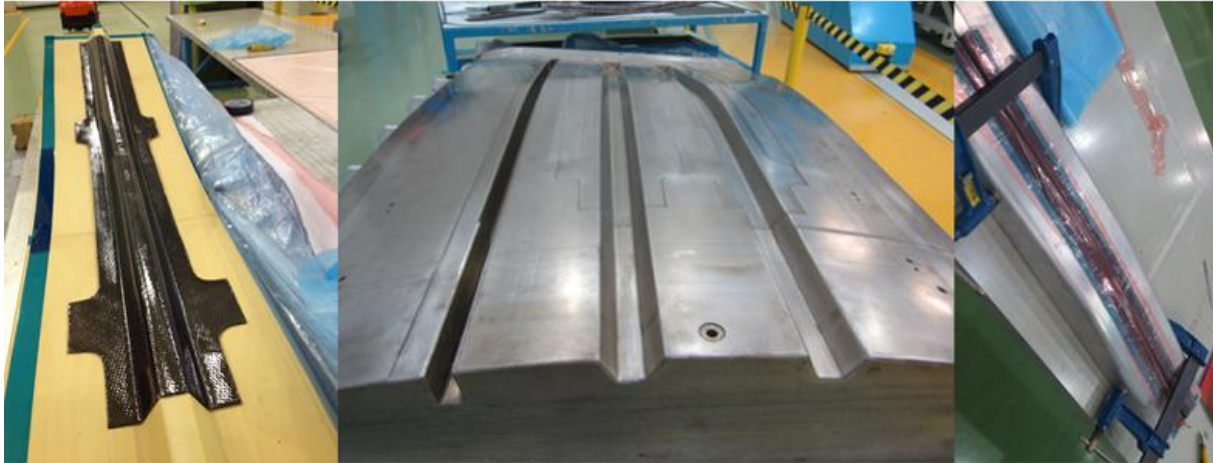
Figure 3. Left) Hot-forming tool for \Omega stringers; mid) integration-curing tool; right) hot-forming tool for T stringer
