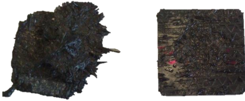
Figure 6: Size reduction of thermosets using high (left) and low (right) voltages at comparable energy input
