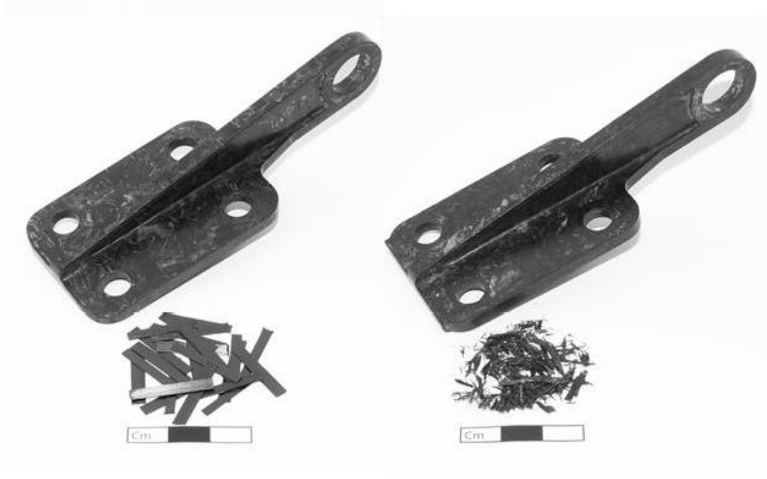
Figure 8: Door hinge processed with chopped tapes and electrodynamic recycled fragments. Pictures provided by M. Roux FHNW, Switzerland).
