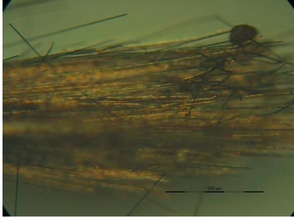
Figure 12: Micrographs to different magnification from C-fibers liberated from thermoset composites by electrodynamic fragmentation. Picture provided by M. Roux, FHNW, Switzerland.
