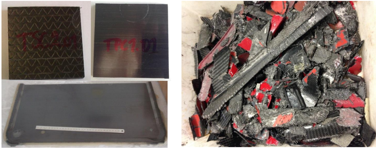
Figure 3: Figure 3: Samples used for the process development. Lab scale tests of WP 1& 2 used upper left in dimension 40x40 mm. Below left was used to test large forms in Plant D setup in WP 3. Right shredder sample was used in WP 3 in plant E setup.
