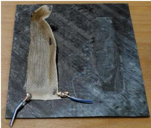
Figure 23 Disassembled omega stringer from skin
