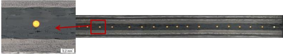
Figure 14 Light optical micrographs of the embedded final design of the separation layer
