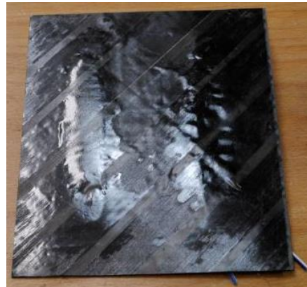
Figure 23 Disassembled omega stringer from skin
