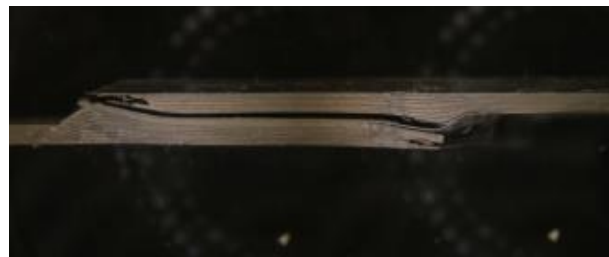
Figure 18 Side view of single lap shear test specimen (without separation layer) with tape undulation
