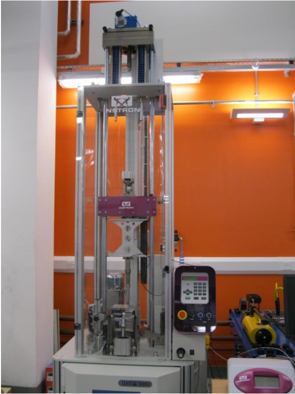
Figure 12: Drop tower used for the validation of passive sensing.
