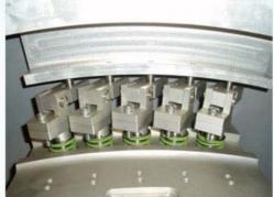
Details of the Variable Inlet Guide Vanes-VIGVs, developed by SENER © The design and manufacturing of the mechanism and the electromechanical actuators was carried out in the OPENAER CENIT project.
