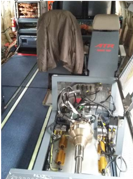
Image 3. Flight-EMA and In-Flight TB performing validation test in the ATR aircraft cabin
