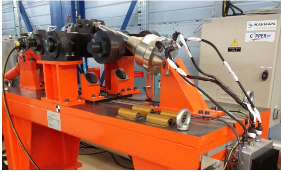
Image 4. Flight-EMA and On-Ground TB performing validation test in Copper-Bird installation at LBS facilities
