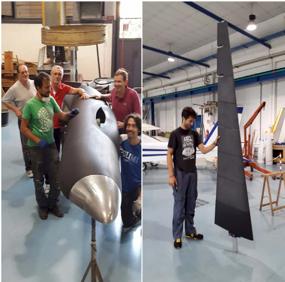
Figure 3: Fuselage and wing during the final assembling.
