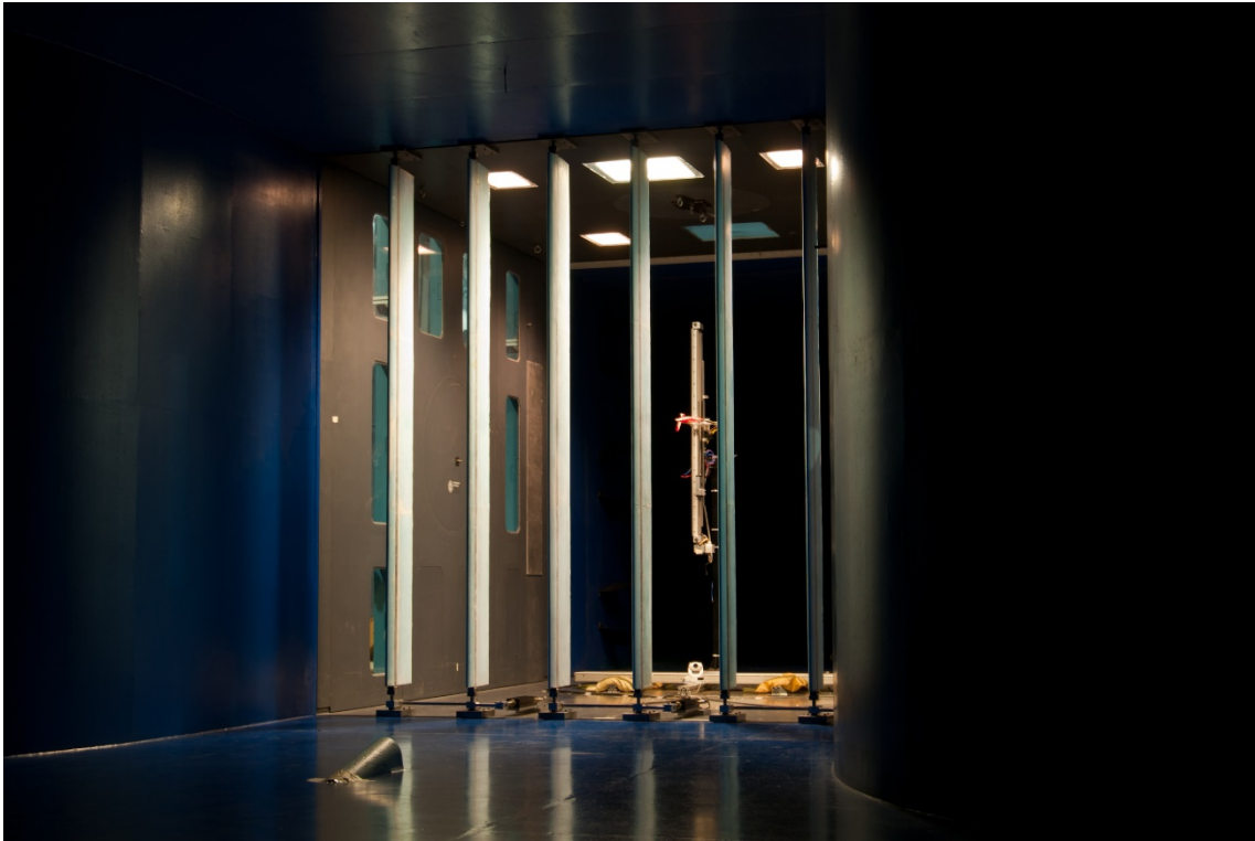
Figure 4: The Gust Generator installed in the wind tunnel during the calibration phase.
