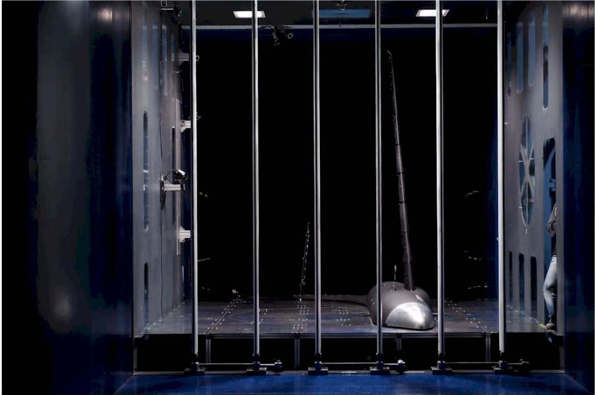
Figure 6: The GLAMOUR model inside POLIMI's wind tunnel ready for gust loads alleviation tests.
