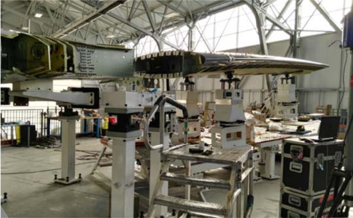
Stage 4 ready for assembly new win with Transition Structure
