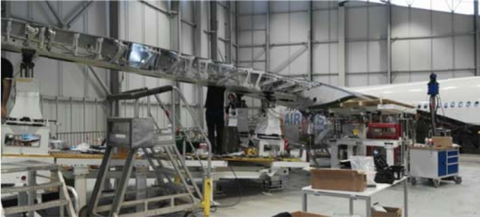
New wing in final assembly position with transition Structure
