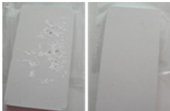
Figure 1: Top view of Mg EV31 sample processed within phosphate containing electrolyte (right) and without phosphate (left)/ J=20\text{A}/\text{dm}^2 , f = 500\text{ Hz} , t=5\text{ min} .
