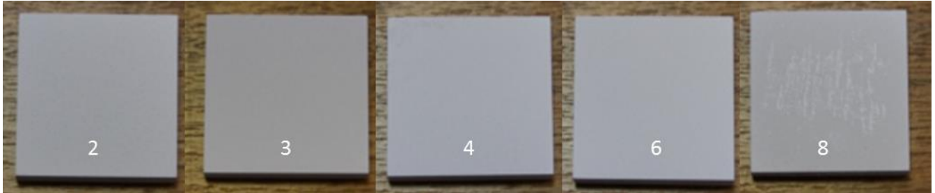
Figure 7: pictures of Mg samples after MAO processing in \text{KOH} + x \text{ g/L Na}_2\text{SiO}_3 . Values of x are indicated in the figures. (100 Hz, 15 min, 40 A)
