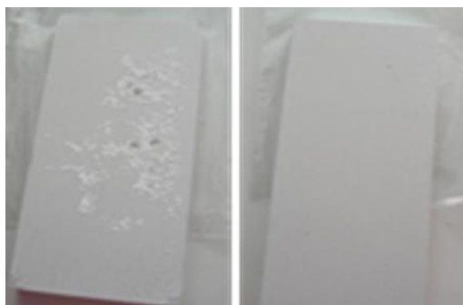
Figure 14: Top view of Mg EV31 sample processed within phosphate containing electrolyte (right) and without phosphate (left) / I=20\text{A}/\text{dm}^2 , f = 500 \text{ Hz} , t=5 \text{ min} .
